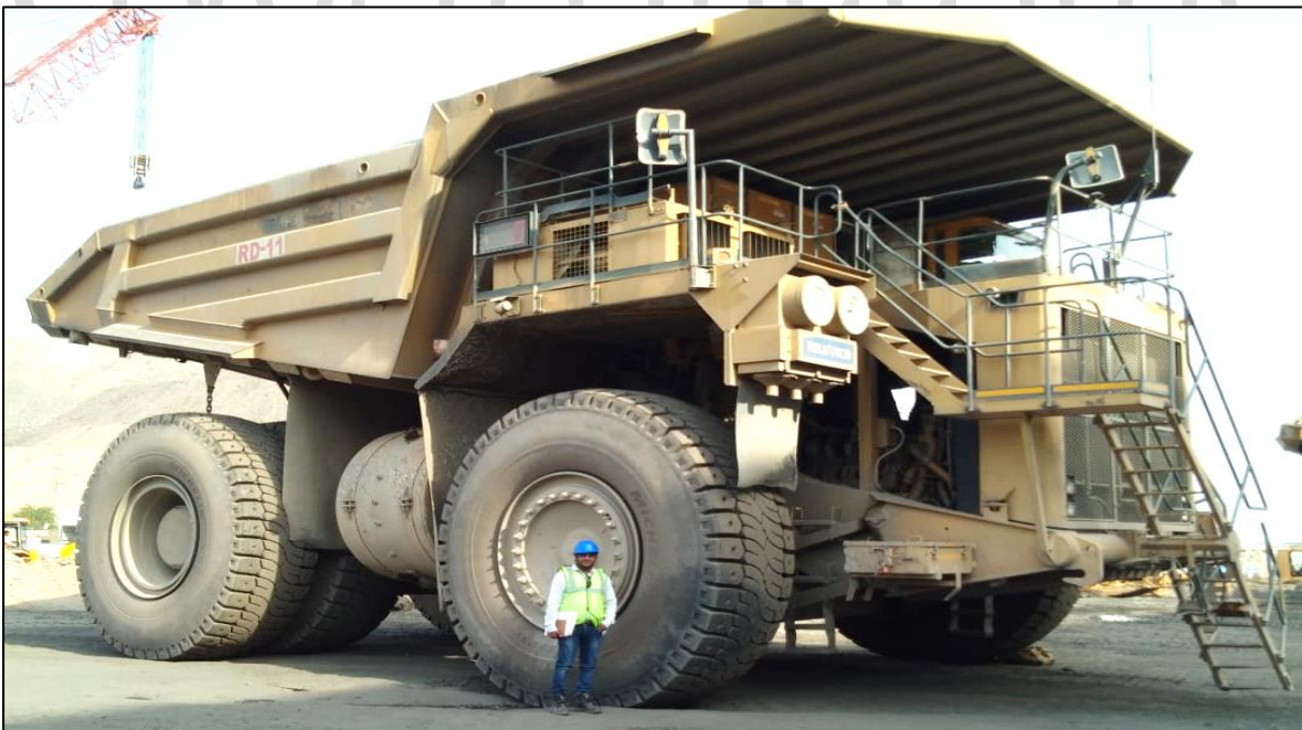
225 MT Payload dumper truck Courtesy : Reliance SASAN Power, Cryogas equipment Pvt Ltd during Site Visit of our LNG Engineer
