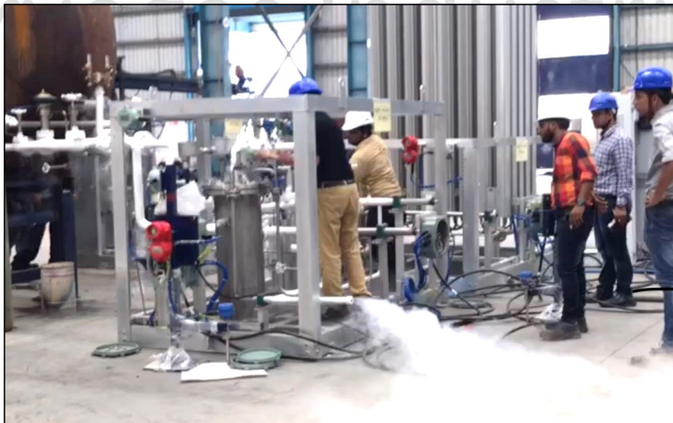
Actual testing picture at Cryogas shop using liquid nitrogen at -196 degc for validation purpose
